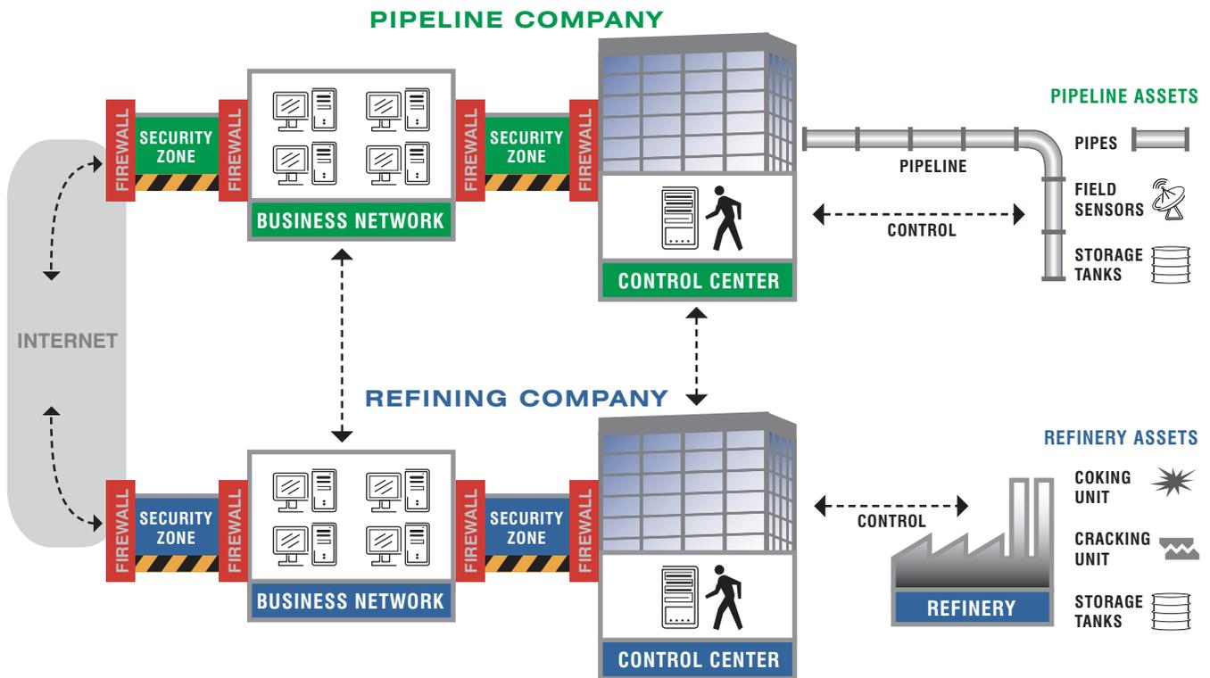
Process control networks are typically separated from the business network by a double-firewalled security zone. The control center monitors and manages a complex network of sensors, which provide real-time data on critical processes. Data may be transmitted to and from the control center via the Internet or other means. Despite security measures, vulnerabilities persist at each point in the communication chain. *(Content provided by A. McIntyre.)*
